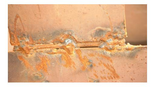
What does an acceptable joint mean? In the above picture we see that the welder has inserted a piece of the welding rod in order to compensate for wrong fit-up and dimensional control, Buttering would be the natural solution for such a joint.
